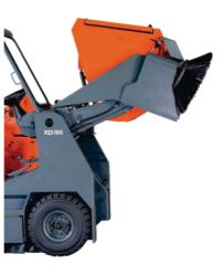
Side broom integrated with the arm - enables riding on bumps and speed breakers easy without any damages.
