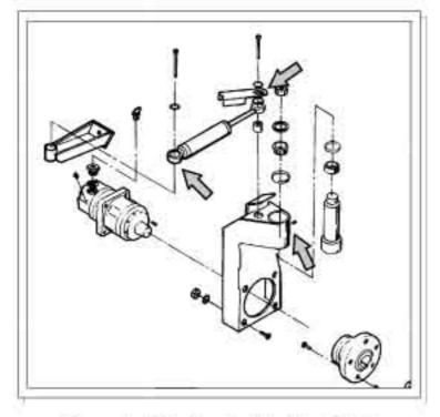
**Powerflex Steering Lubrication Points**
