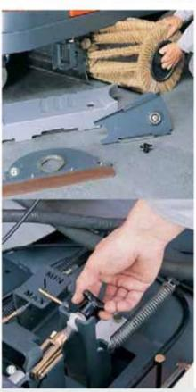
The central sweeping level adjustment, which can be adjusted without tools, guarantees correct, even pressure of the suspended main broom.
