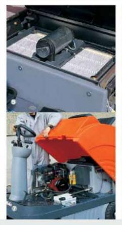
The clearly laid out engine compartment is easily accessible for servicing and maintenance purposes via the seat console, which simply tilts backwards.
