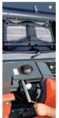
Objects, foils or tapes which are difficult to sweep up can be thrown through the waste container flap without having to open the container itself and without causing any dust to escape . The waste container can be lifted via the hydraulic raising attachment and emptied at any height ...
