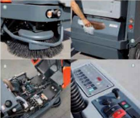
The Jonas 1500 cockpit can be accessed easily from both sides. Clear view of the side brushes at the front. The particularly simple operating concept ensures the user does not get confused. The entire sweeping function can be switched on and off with just one button
